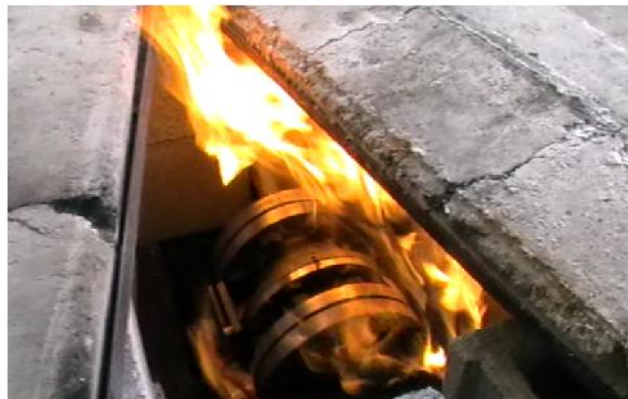
Valves under functional and endurance test for steam service
