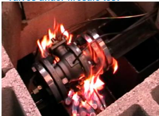
Valves under firesafe test
