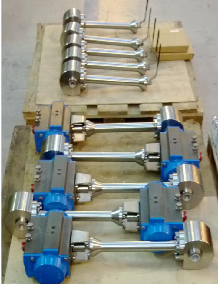
Application: LNG (for gas filling stations), Delta P 240Bar, circa 60,000 cycles/year
